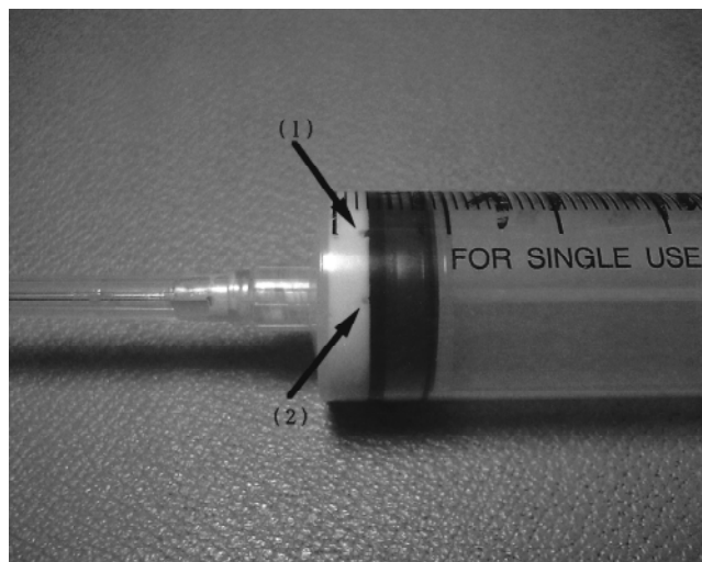
Fig. 1. Rubber fragment and air bubble in the propofol syringe. A rubber fragment that is close to the piston of a syringe is potentially mistaken for an air bubble. (1) Air bubble, (2) rubber fragment
